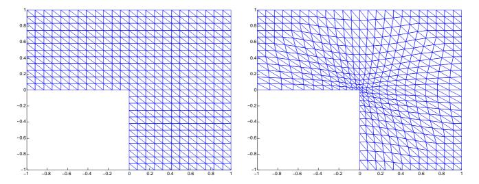
Figure 2: Triangulation of an L-shape for  $\nu = 12$ . On the left we find the uniform triangulation, and on the right its image under the map  $\phi(x) = x \cdot \min\{1, \sqrt{||x||}\}$  leading to some grid refinement around the origin.
