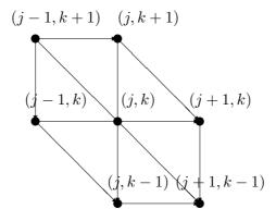
Figure 1: The vertex (j, k) and its adjacent vertices for  $P_1$  Finite Elements.
