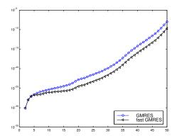
Fig. 5.2. Orthonormality of the Arnoldi vectors for Example 5.1:  $||I_k - V_k^* V_k||^2$  as a function of k for Algorithm 4.4 (symbol  $\triangleright$ ) and standard GMRES (symbol  $\circ$ ).
