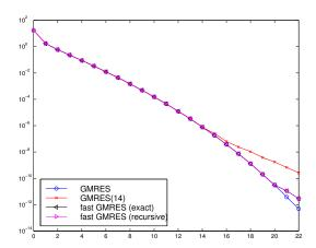
Fig. 5.5. Residual norms for Algorithm 4.4 applied to the data of Example 5.3. For comparison, we display both the norm of the exact residuals  $||b - Ax_k||$  (symbol  $\lhd$ ) and the recursive residual norms  $|\gamma_k|$  (symbol  $\rhd$ ), which are of the same size, and slightly smaller than those obtained for restarted GMRES(14) (symbol  $\times$ ). The norms of the residuals  $r_k'$  determined by standard GMRES (symbol  $\circ$ ) are somewhat smaller for  $k \geq 21$ .
