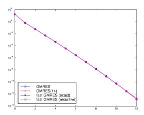
Fig. 5.3. Residual norms for Algorithm 4.4 applied to the data of Example 5.2. For comparison, we show both the norm of the exact residuals  $||b-Ax_k||$  (symbol  $\lhd$ ) and the recursive residual norms  $|\gamma_k|$  (symbol  $\triangleright$ ), which are of the same size. The norm of the residuals  $r_k'$  obtained by standard GMRES (symbol  $\circ$ ) and by restarted GMRES(14) (symbol  $\times$ ) are also displayed.
