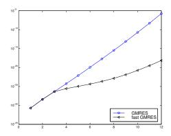
Fig. 5.4. Orthonormality of the Arnoldi vectors for Example 5.2:  $||I_k - V_k^* V_k||^2$  as a function of k for Algorithm 4.4 (symbol  $\triangleright$ ) and standard GMRES (symbol  $\circ$ ).
