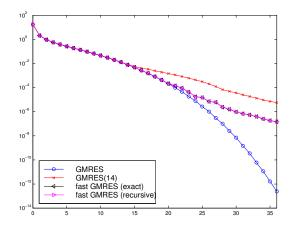
Fig. 5.7. Residual norms for Algorithm 4.4 applied to the data of Example 5.3. For comparison, we show both the norm of the exact residuals  $||b-Ax_k||$  (symbol  $\lhd$ ) and the recursive residual norms  $|\gamma_k|$  (symbol  $\rhd$ ), which are of the same size, and smaller than those obtained by restarted GMRES(14) (symbol  $\times$ ). The norms of the residuals  $r_k'$  obtained by the standard GMRES (symbol  $\circ$ ) are much smaller for  $k \geq 30$ .
