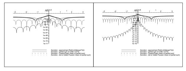
Figure 3: The modulus of the error of approximation on a logarithmic scale of the Fourier series of  $f(t) = |\sin(\frac{t}{2})|$ . On the left we use the first 7 and on the right the first 17 coefficients of the Fourier series.
