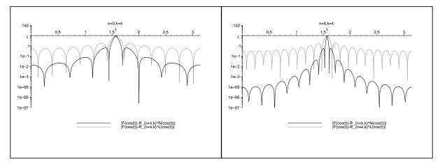
Figure 2: The modulus of the error of approximation on a logarithmic scale at  $x = \cos(t)$  of the linear and the nonlinear Padé-Chebyshev approximant of  $F(x) = \operatorname{sign}(x)$ .
